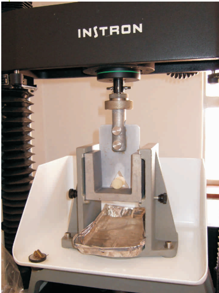
Universal Testing Machine (Instron 4500) used to determine shear values of potato samples.
