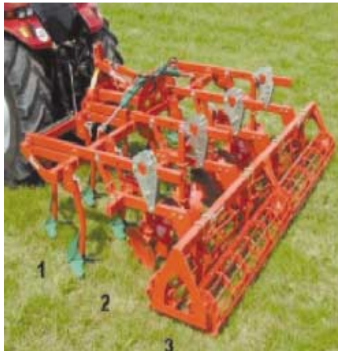
Figure 3. Combine cultivation steps to decrease field traffic: 1 - loosening and mixing; 2 - leveling; 3 - compacting and breaking clods.
